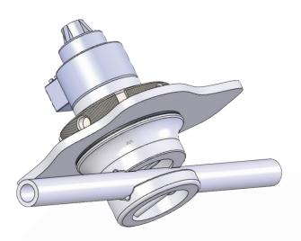
Clippard's PPV series pinch valve proportionally controls the flow of liquids and gases by pinching a tube set using a high force, high accuracy stepper-driven linear actuator. Its unique design features enable you to take your applications to the next level by providing proportional resolution and linearity that far exceed those of competing models (see chart below).
